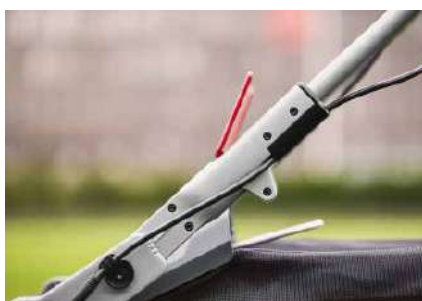
Foldable handle to reduce space for storage (82LM46SX and 82LM51SX).
