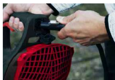
Cable connection of the 82B20 to connect the battery.
