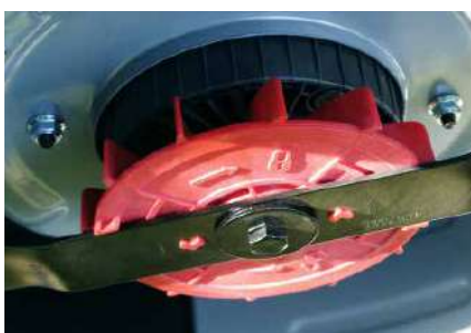
Fan for increased turbulence and cooling of motor.
